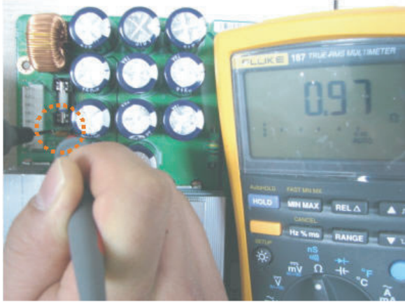
Ve fuse (F4005) – OK (0.x ~ x.x ohm)
