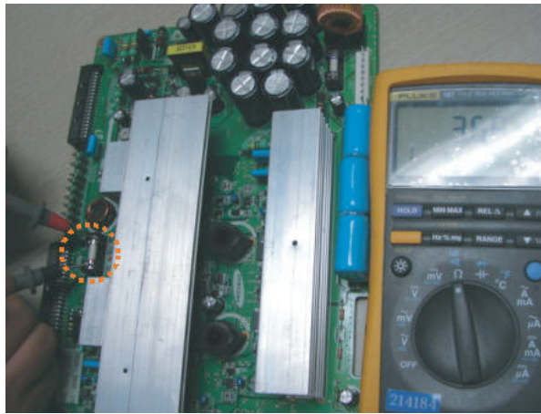
Vs fuse (F5006) – OK (0.x ~ x.x ohm)
